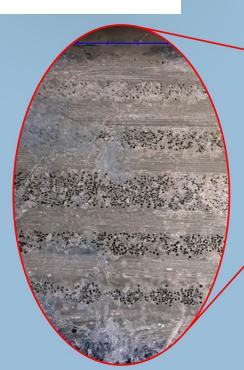
With a center closed cell foam and finely placed unidirectional fibers at 0° and 90°, the composite material includes multiple layers across the entire one-piece construction.
